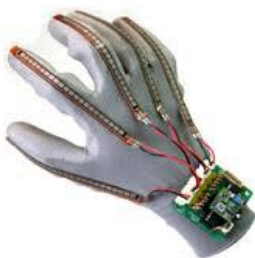
Figure 3: Data glove with flex sensor
