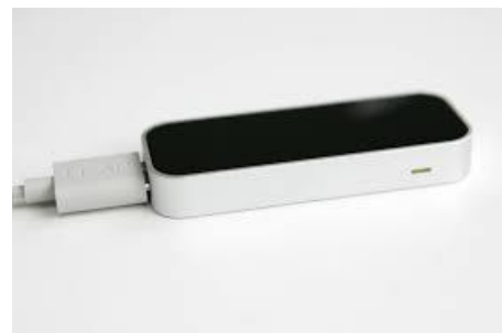
Figure 1: Leap motion controller with USB
