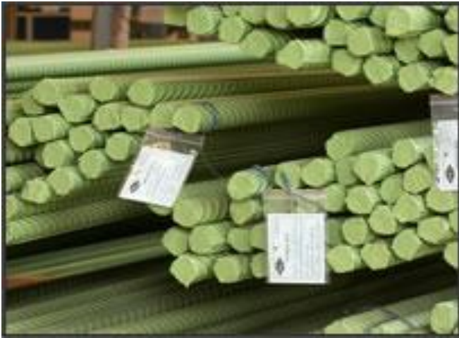
Epoxy coats rebar
