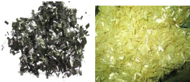
Figure.11: Reinforced fibers chopped carbon and short Kevlar fiber used for epoxy composite system
