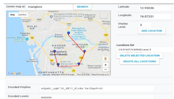
Figure 5: interactive polyline encoder utility algorithm for managing bus stops
