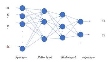
Every circle in the above network represents a neuron at which the inputs and corresponding weights are processed layer by layer.
