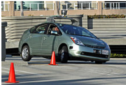
A Toyota prius modified to operate as a Google driverless car, navigating a test course.
