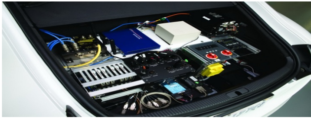
On board computers of Stanford/Audi autonomous TTS
