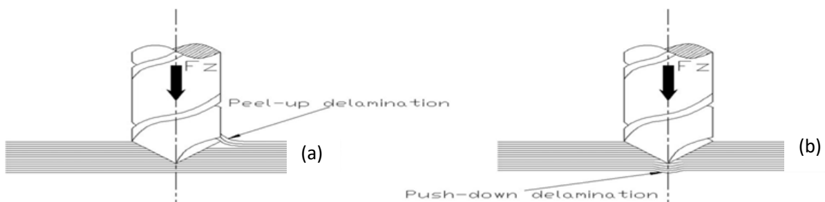
Fig. 2. (a) Peel-up delamination (b) Push-down delamination (From, Amrinder PS, Manu S, Inderdeep S. A review of modeling and control during drilling of fiber reinforced plastic composites. Compos Part B Eng. 2013; 47: 118–25. Reproduced with permission of Elsevier)
