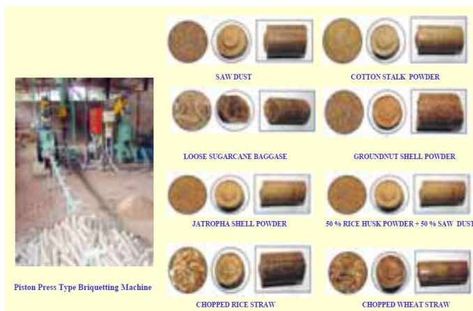
Fig. 6 Different Types of Feedstock for Piston Press Type Briquetting Machine
