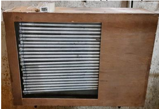
Figure 6: Waste Heat Recovery System with Composite PCM inside Aluminum Tubes
