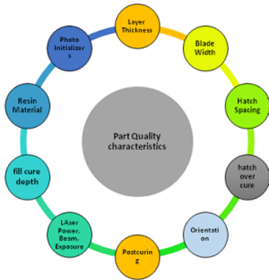
Figure 5 Process Parameters of SLA
