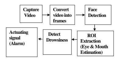
Fig 2: Block diagram of Drowsiness Detection System
