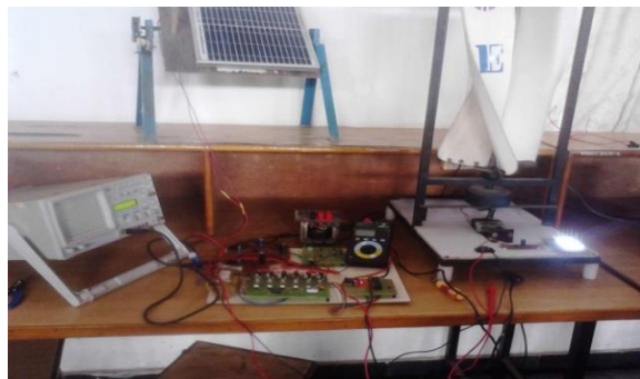
Fig (15): Experimental setup of Renewable hybrid wind solar energy system fed single phase inverter. Hardware results:
