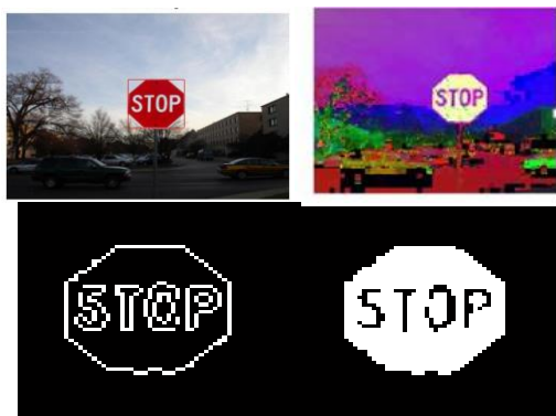
Fig 7: Detection process of a stop sign
