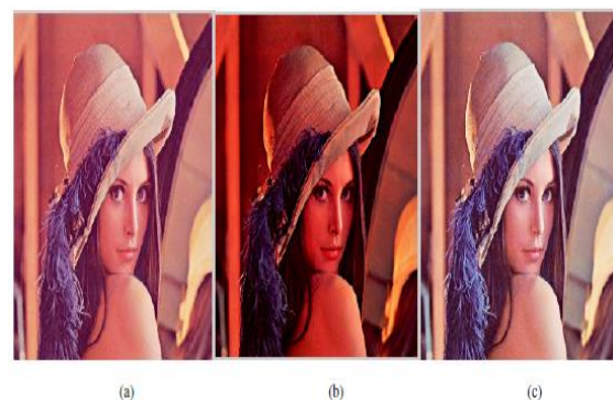
Fig1: (a) original image (b) Enhanced image by using HE (c) Enhanced image using HM
