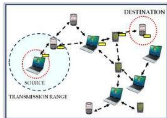
Figure 1: Infrastructure-less or Mobile Ad-hoc Network
