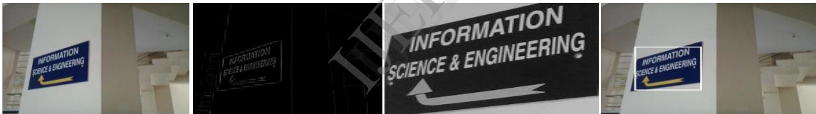
Fig. 6. Example on the oriented text region localization (from left to right: original images, results of background suppression, merging of text blocks and text region localization)
