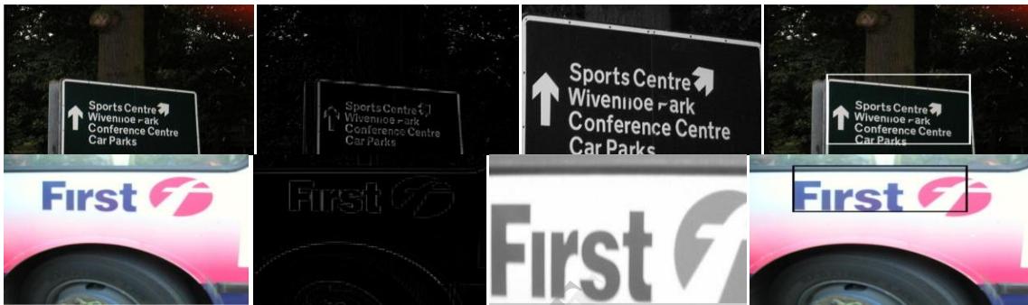
Fig. 5. Text region localization examples on the ICDAR 2011 competition dataset (from left to right: original images, results of background suppression, merging of text blocks and text region localization)
