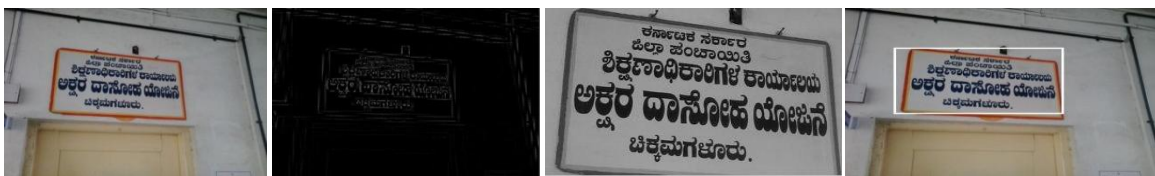
Fig. 7. Example on the Kannada text region localization (from left to right: original images, results of background suppression, merging of text blocks and text region localization)
