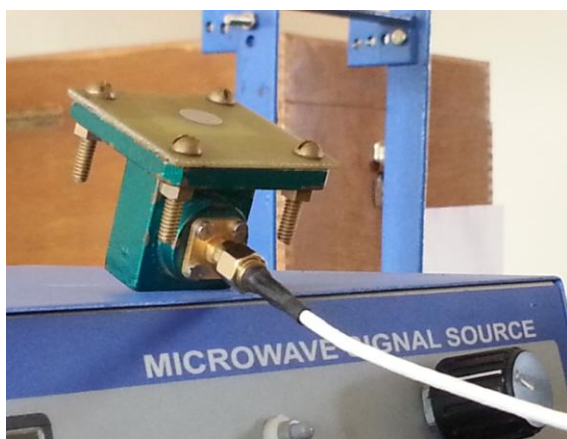
Fig.7. Mounting of Waveguide Coupled Microstrip Patch Antenna to waveguide to coaxial adapter.
