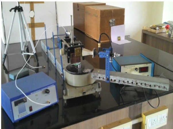
Fig.3. Experimental setup for Radiation Pattern measurement.
