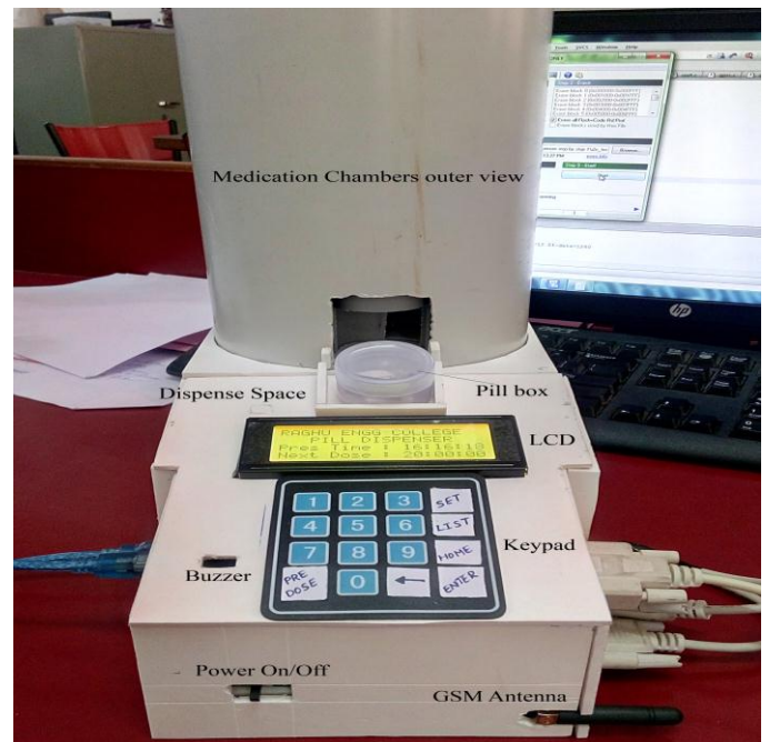
Fig. 4: Prototype of Automated Medication Dispenser
