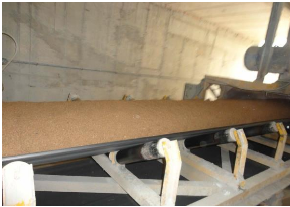
Figure 6. Conveyor feeding sand to the mixer
