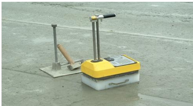
Figure 18. Nuclear experimental apparatus for measuring density
