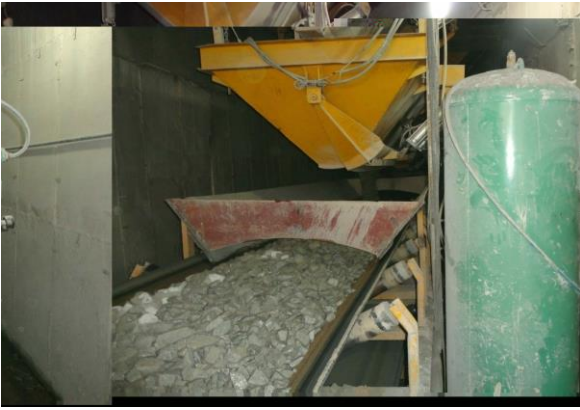
Figure 5. Conveyor feeding rocks to the mixer
