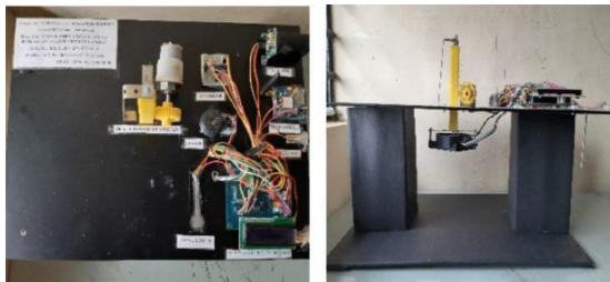
Figure 7: Photograph of a Ceiling Fan Based System to Avoid Suicide by hanging system prototype.
