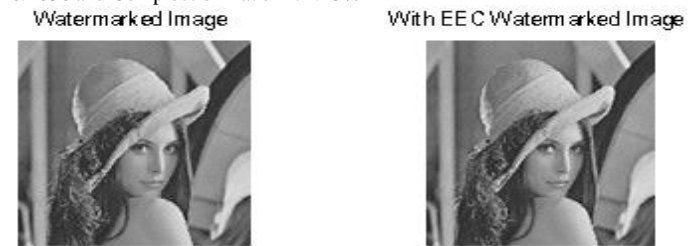
Fig. 8(g). Watermarked image with Error Correcting code (Cyclic Code) with PSNR = 58.5615 dB and Compression Ratio = 71.1594%
