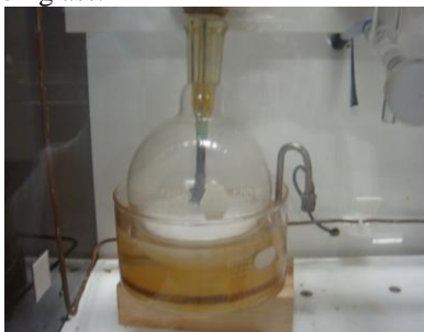
Figure 2. Oil sample placed in discharge cell according to ASTM Designation D6180
