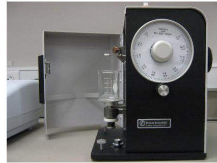
Figure 6 . Tensiometer For interfacial tension (IFT) measures [6]
