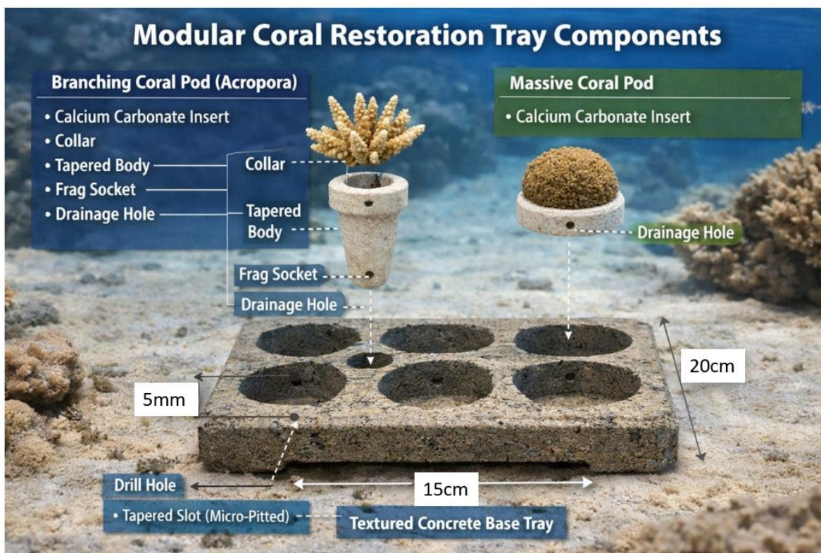
Figure 2 Exploded view of the system components, illustrating the base tray and individual \text{CaCO}_3 inserts. Key features include tapered geometry for secure seating, a central socket for coral fragment placement, and a drainage aperture to facilitate water exchange.
