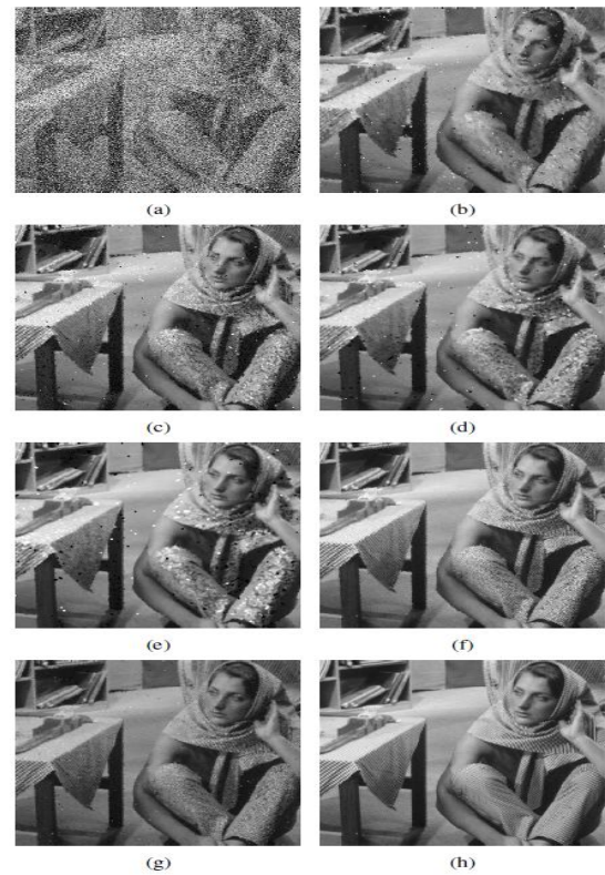
Fig.2. Performance of different filters for "Barbara" image with 50% salt and pepper noise. (a) Noisy. (b) SD-ROM. (c) ACWM. (d) ASWM. (e) DWM. (f) NSWM. (g) Proposed and (h) Original.
