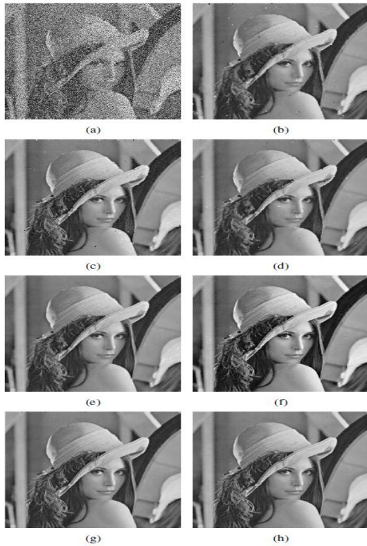
Fig.1. Performance of different filters for "Lena" image with 40% salt and pepper noise. (a) Noisy. (b) SD-ROM. (c) ACWM. (d) ASWM. (e) DWM. (f) NSWM. (g) Proposed and (h) Original.
