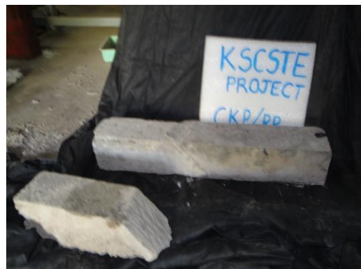
Figure 6 (a) Substrate and repaired beam
