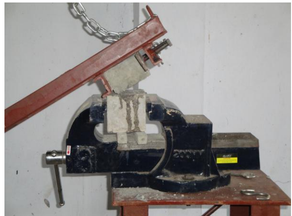
Fig. 4. Specimen after bond failure
