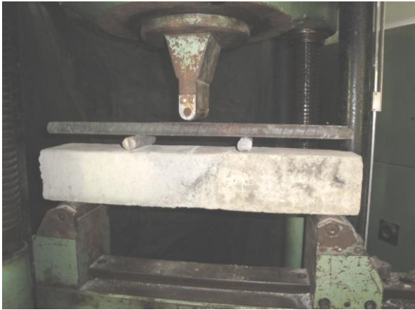
Fig.6(b) Flexure test on repaired beam
