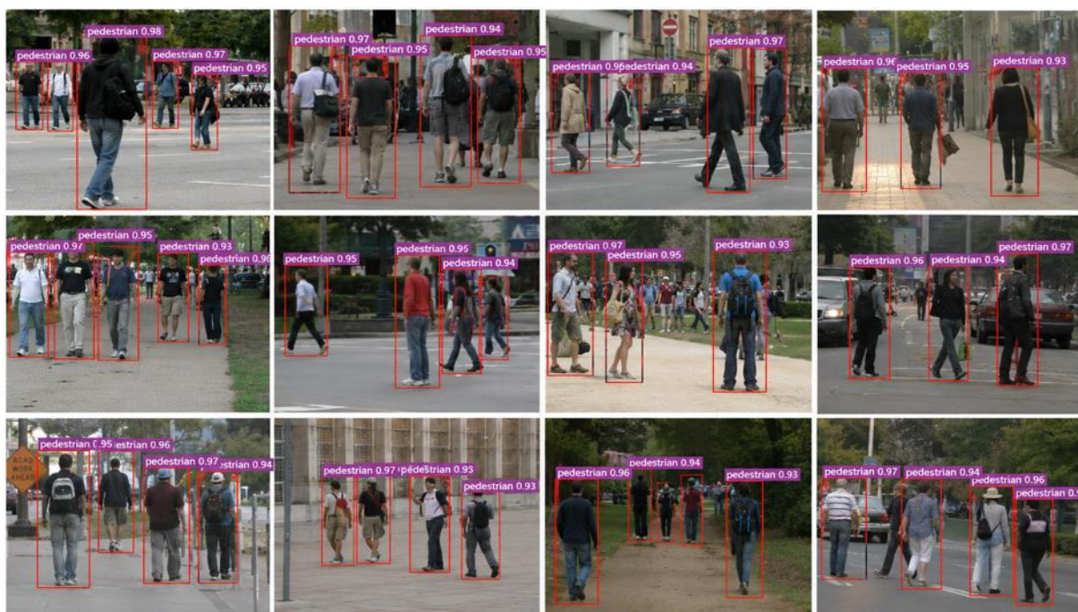
Fig. 7. Qualitative pedestrian detection results of the proposed lightweight attention-based framework on the Caltech Pedestrian Dataset, demonstrating accurate localization and high-confidence detection across diverse urban scenes and pedestrian densities.
