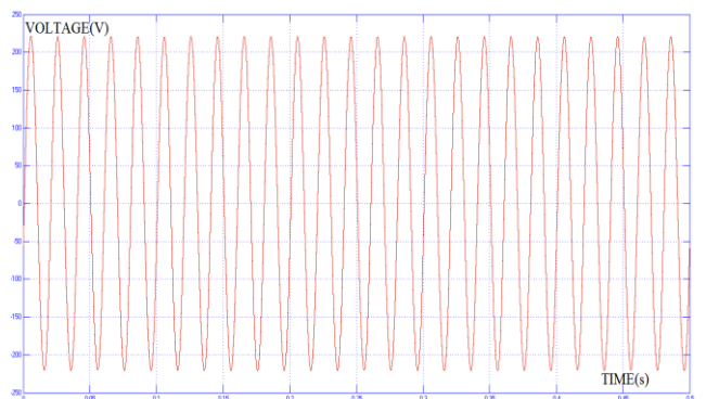
Fig 11 The stimulated result of the inverter side voltage
