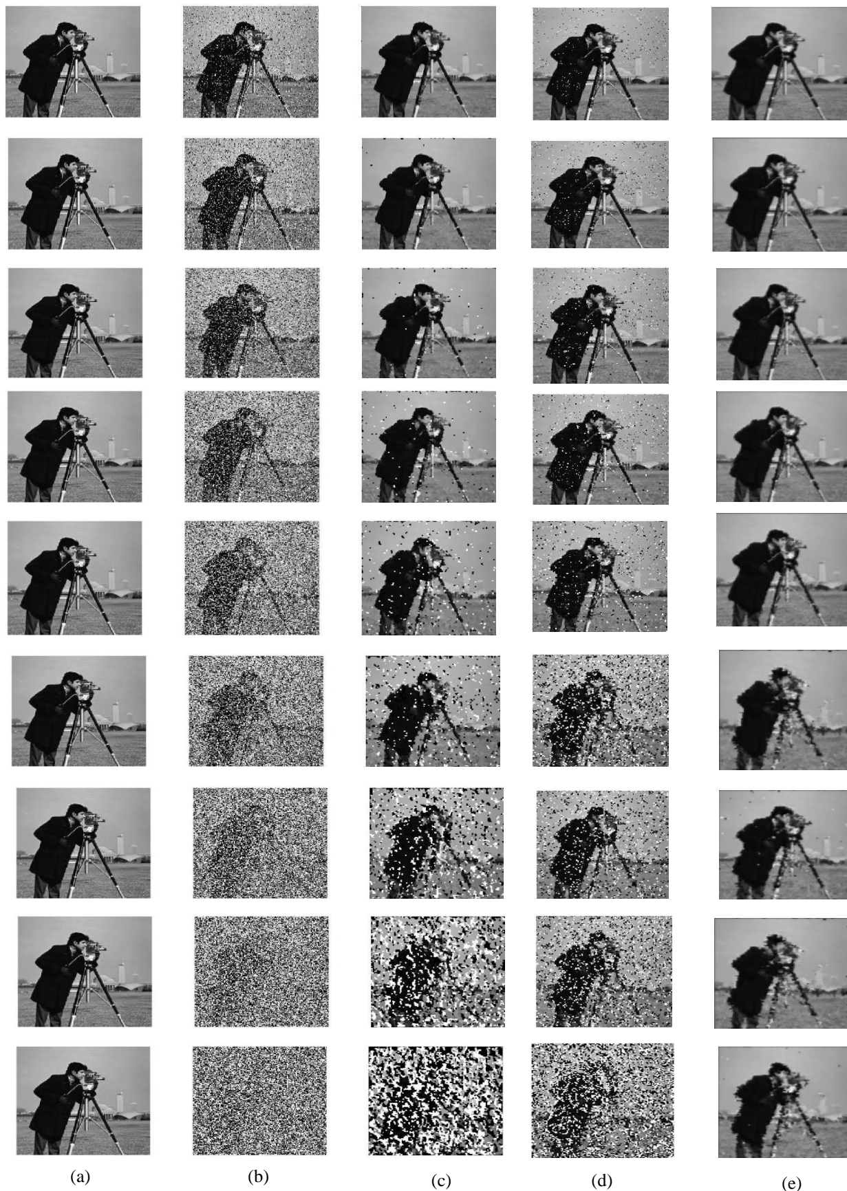
Fig.4 (a) original image (b) noisy image (10% to 90% from top to bottom) (c) recovered image by MF technique (d) recovered image by AMF technique (e) recovered image by Proposed algorithm.
