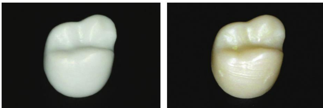
(a) Fabricated by 3D printing (b) Fabricated by subtractive manufacturing
