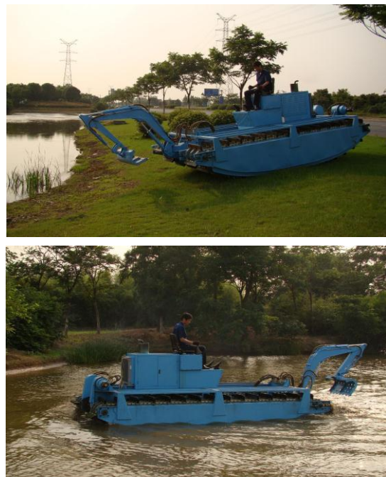
Fig.8 The implementation of the amphibious walking device
