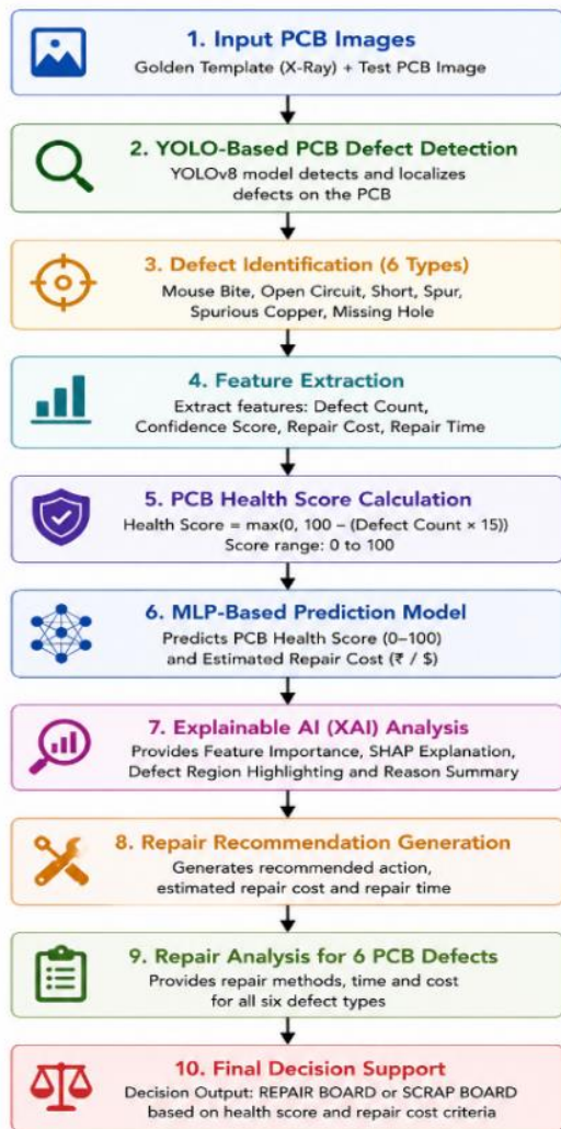
Fig. 1. Proposed Cost-Aware Intelligent PCB Defect Inspection System Workflow.
