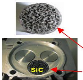
Fig.1 View of PM-engine head and SiC reactor
