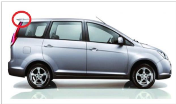
Fig.2: MPV with Spoiler (Proton Exora)
