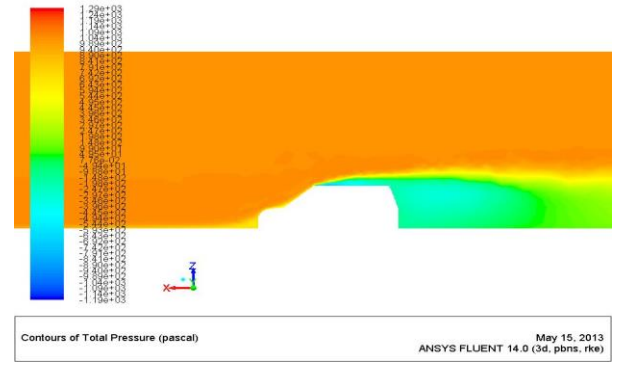
Fig. 13: Contours of Total Pressure (MPVs)
