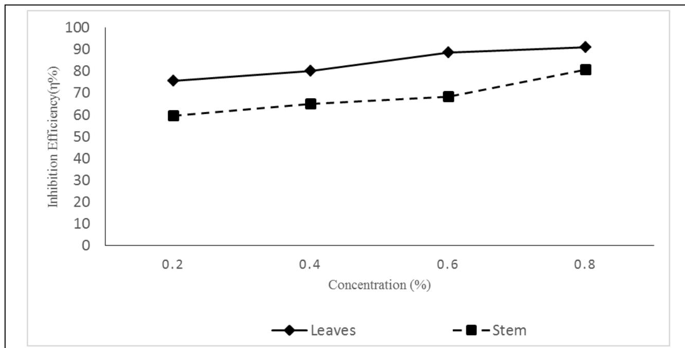
Fig 2 - Variation of Inhibition efficiency as a function of concentration in the presence of different concentrations of *Solanum xanthocarpum* in 2N HCl Solution on Aluminium by Gasometric method
