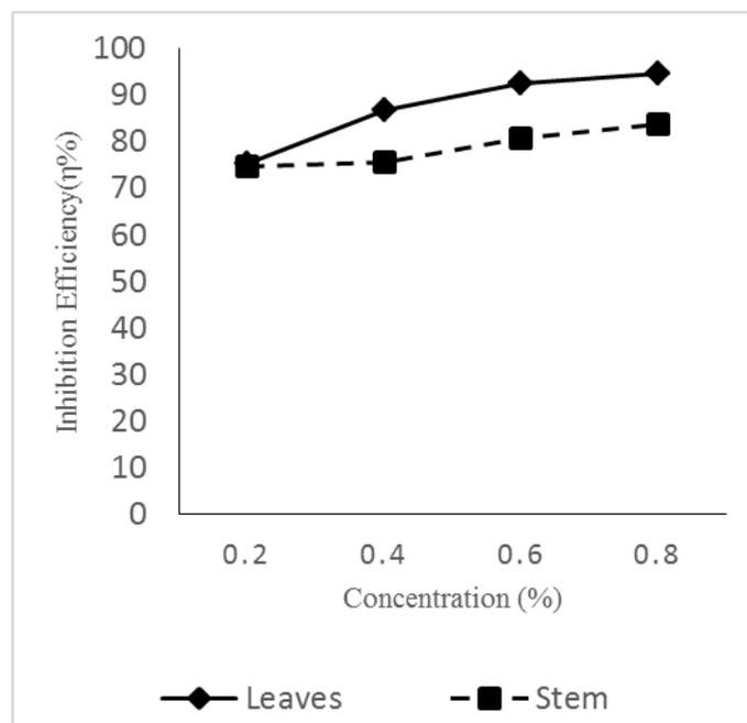
Fig 1 - Variation of Inhibition efficiency as a function of concentration in the presence of different concentrations of *Solanum xanthocarpum* in 2N HCl Solution on Aluminium by weight loss method
