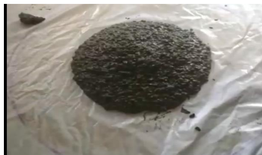
Fig 4 Slump test with 0.75% coir fibre
