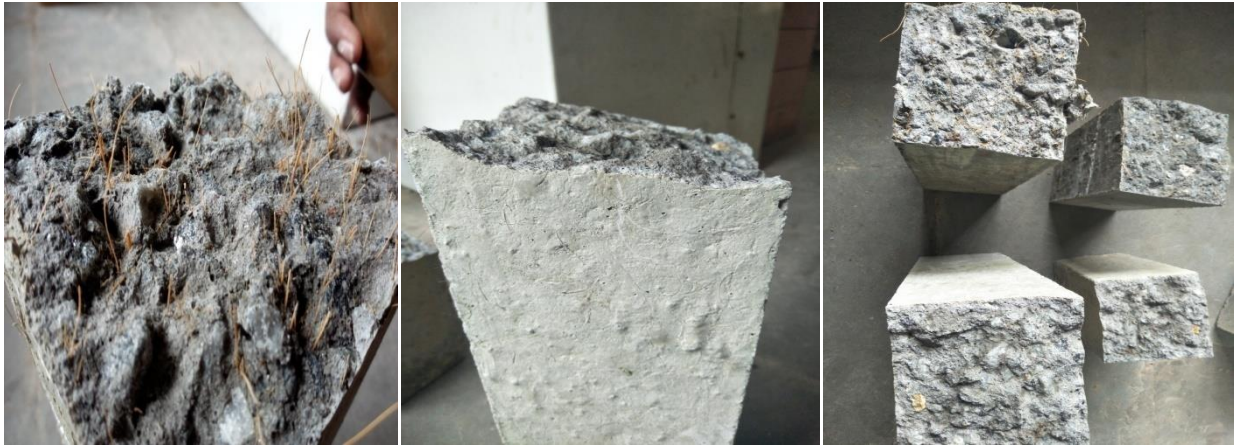
Fig 10 Typical failure patterns for concrete prisms after flexural loading.
