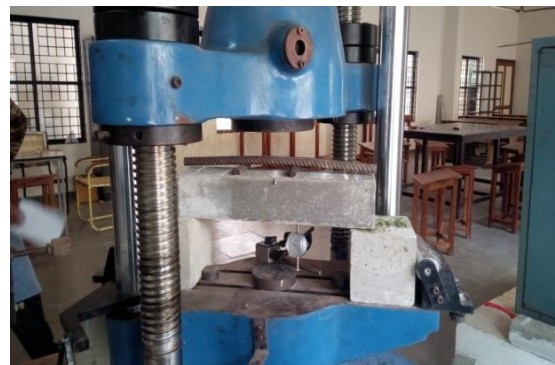
Fig 2 Test set up for Flexural studies
