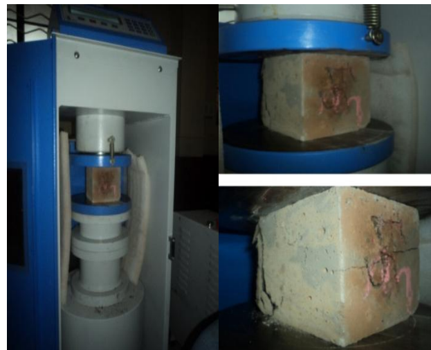
Fig 3: Compressive Strength Test on Cubes
