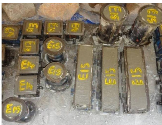
Fig 1: Concrete placed in moulds
