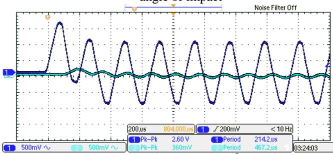
Fig 12.Experimental traces of aluminium for 40<sup>0</sup> angle of impact
