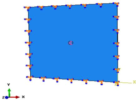
Fig.5 Model of sheet metal after application of boundary condition and load
