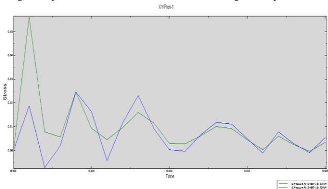
Fig 13.Numerical traces of aluminium for 40<sup>0</sup> angle of impact
