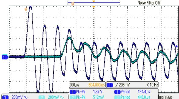
Fig 6. Experimental traces of mild steel at 60° angle of impact
