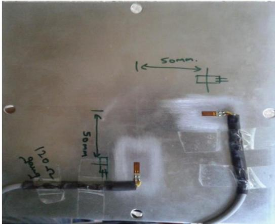
Fig 1. Strain gauges mounted on Sheet metal
