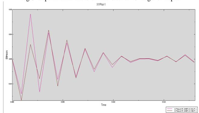
Fig 9. Numerical traces of mild steel at 40° angle of impact
