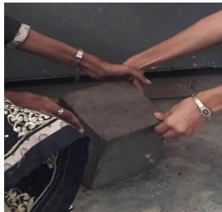
Figure 6 Demoulding of Concrete
