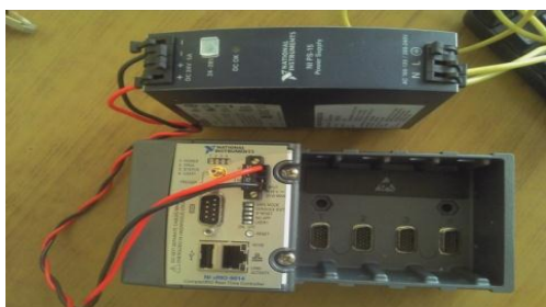
Fig. 5 :CompactRio real-time controller
