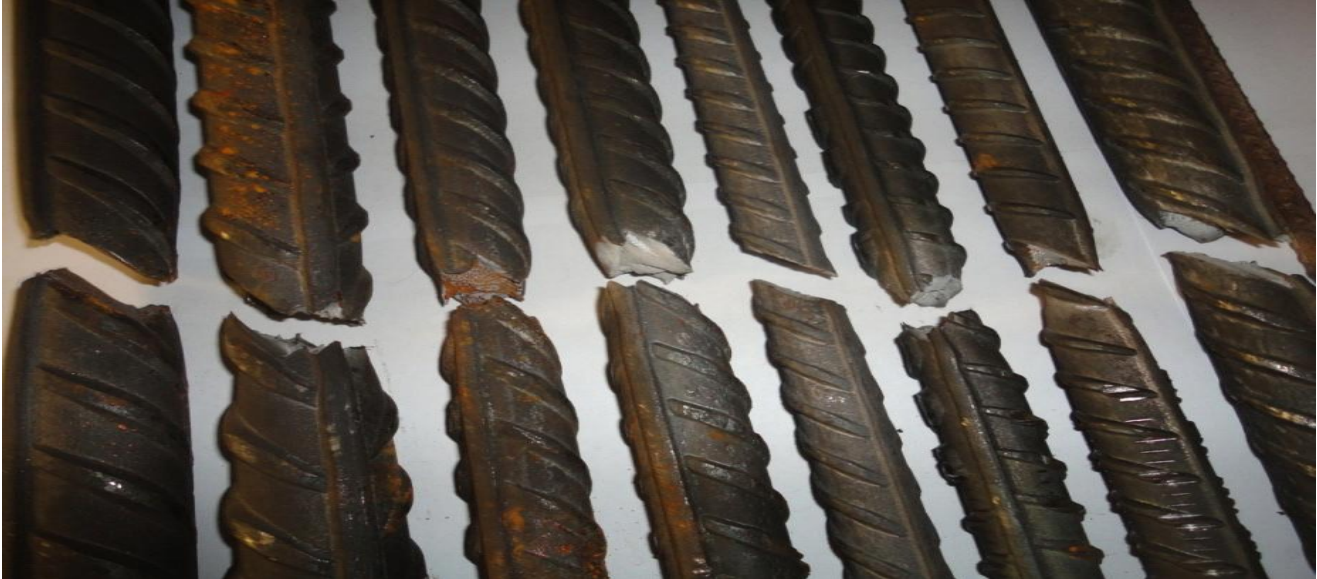
Plate II: Some Broken Test Specimens after Tensile Tests
