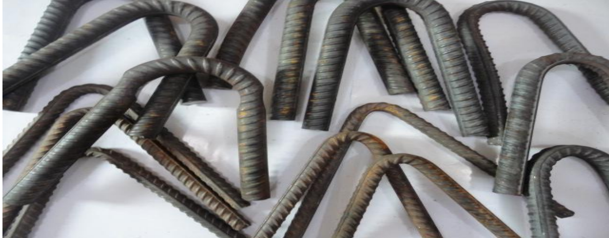
Plate I: Some Test Specimens after The Bend Tests.
