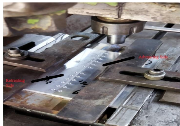
Figure 3 Frictions Stir Welding Fixture Setup and Welding Tool
