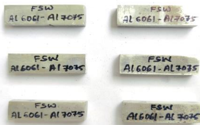
Figure 6 Wear Specimens of Al7075 and Al6061 Species
