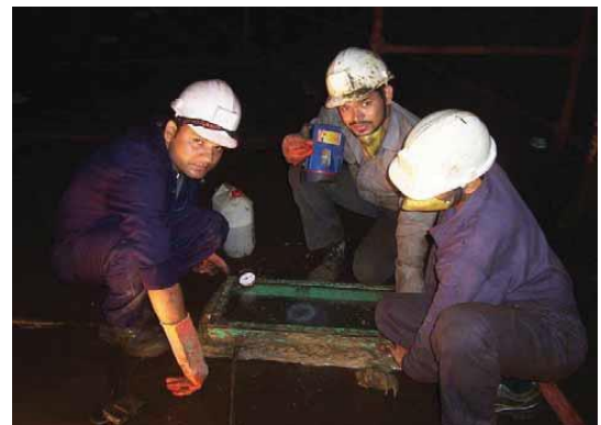
Fig 19. Vacuum Box testing
