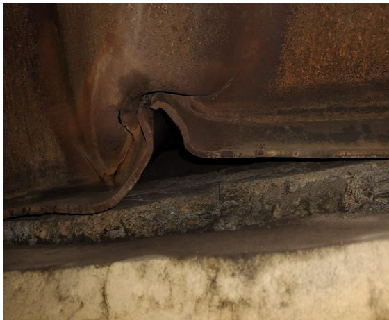
Fig 6. Fracture at Bottom to shell joint
