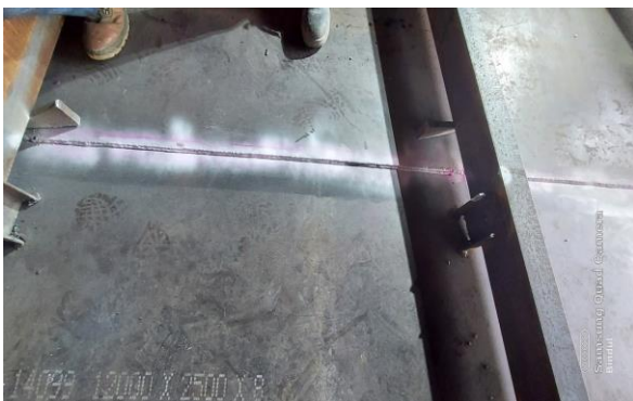
Fig 15. DP test of welding joints
