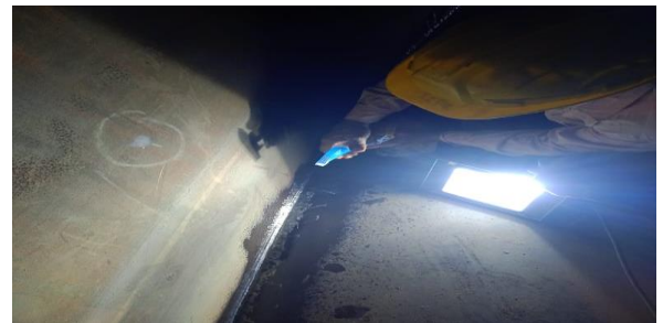
Fig 17. Diesel chalk test of bottom to shell joint
