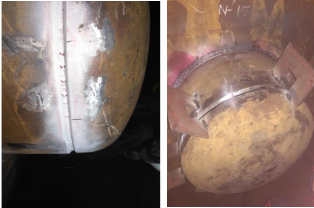
Fig 25. Dished End- Main Manhole welding & Inspection
