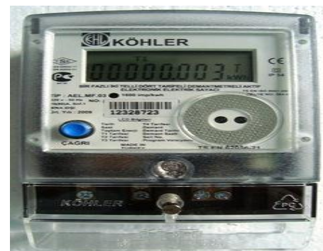
Fig. 2. New electric digital electric meter
