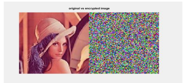
Fig 5. Secret image before and after xor operation with randomly generated image at level 2.
