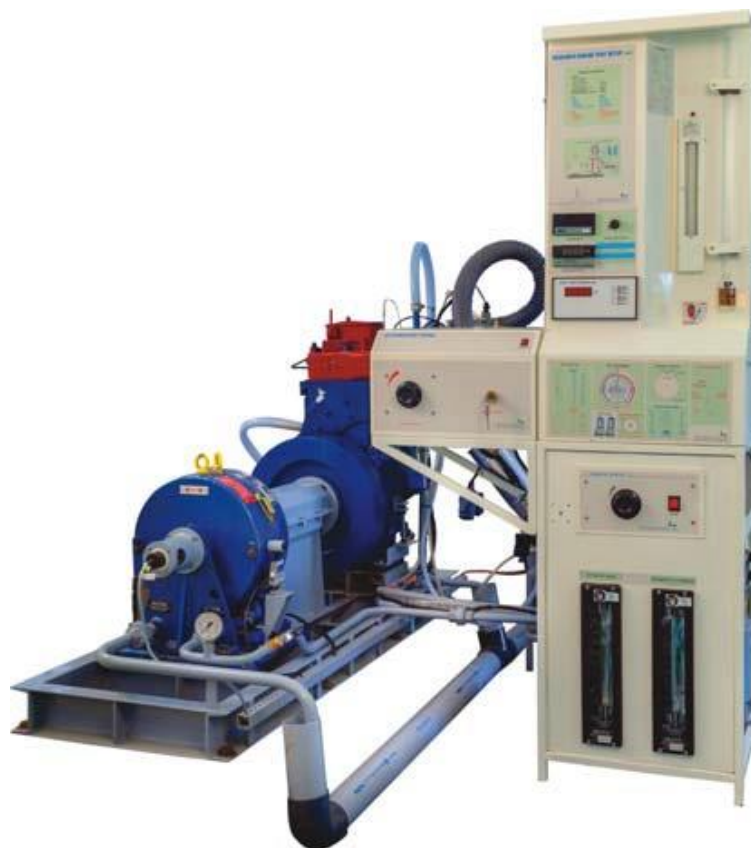
Single cylinder, four stroke, VCR (Variable Compression Ratio) Research engine
