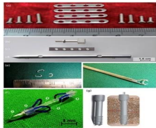
Figure 3: Mg-based biomedical devices are shown in Fig. 3: (a) Biodegradable magnesium bone implants [38]; (b–d) orthopaedic fixation components, (e) pure magnesium microclips used in laryngeal surgery [25]; (f) surgical sutures [26]; and (g) additional medical instruments and dental applications [27].
