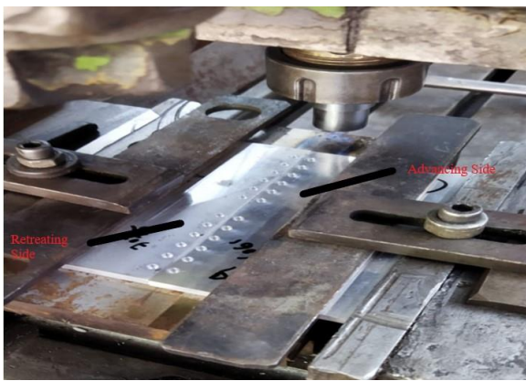
Figure 2 Frictions Stir Welding Fixture Setup and Welding Tool
