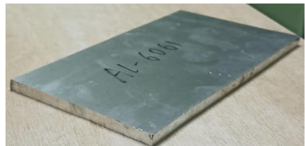
Figure 1 Base plates of Al6061 and Al7075 were machined to specified dimensions
