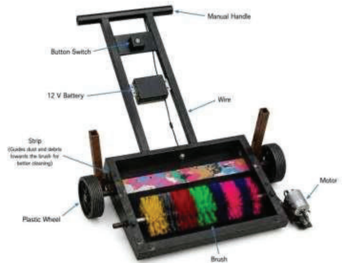
Fig. 7: Fabricated Improved Mechanized Manual Floor Sweeper
