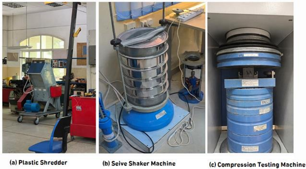
Fig. 3. Equipment used in this study: (a) single-shaft plastic shredder; (b) mechanical sieve shaker for gradation analysis; (c) compression-testing machine.
