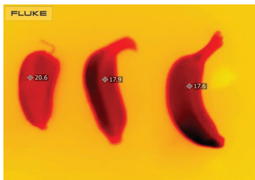
Fig-3 Bananas in Thermal Camera (The varying ripeness is depicted in different temperature ranges)
